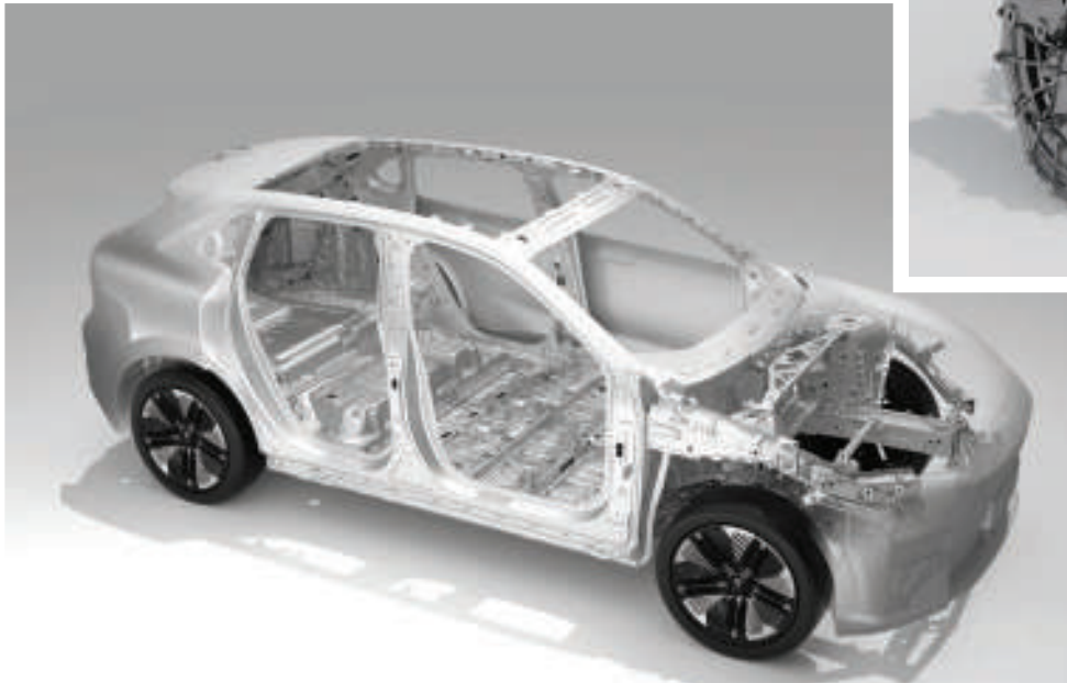
EPA1 PLATFORM WITH HIGH STRENGTH STEEL AND ALUMINUM ALLOY CHASSIS
